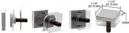
The secondary cap, with removable Allen screw, has two flat sides which are used to secure the cap to the panel material. When firmly in place, the top cap is paced over the secondary cap, then aligned with the square base and held in position with undetectable double-sided tape. With this design there is no "adjustment" or "trial-and-error" required to line up the cap with the base. Requires a 5/8" hole for assembly.
